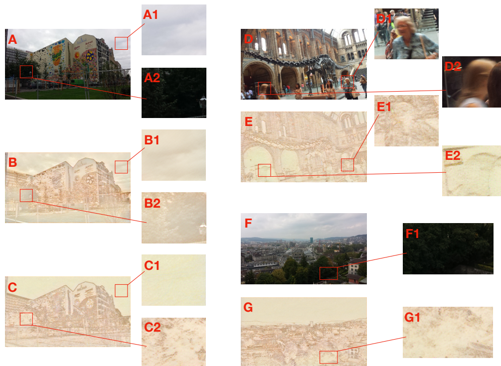
Figure 10: Some little defects. Here we mainly have two defects. One is shown as image C2, E1, E2 and G1, which can be concluded as detail loss. The other is presented in image C1, which can be concluded as object loss. The previous one can be attributed to the mistiness of the input image (see A2, D1, D2 and F1). While the latter one is a shortage of the image preprocessing techniques. We can see that the result with grey-scale input B performs better with both the clouds(B1) and the tree(B2). However, the problem is again the color. Till ddl, we are still not sure why a grey-scale input content can lead to a color like green(B2). Nevertheless, we still choose images like C to be our final results. (see Figure 1)
